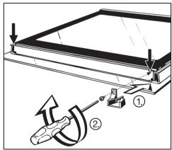
■ Put the guides back in position, then tighten the screws in the trim.
